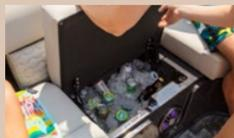
(2) Bow Coolers Integrated into Fiberglass Seat Bases
